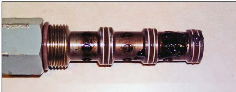
Figure 3: Varnish Found on Fuel Oil Stop Valve Pilot Spool
